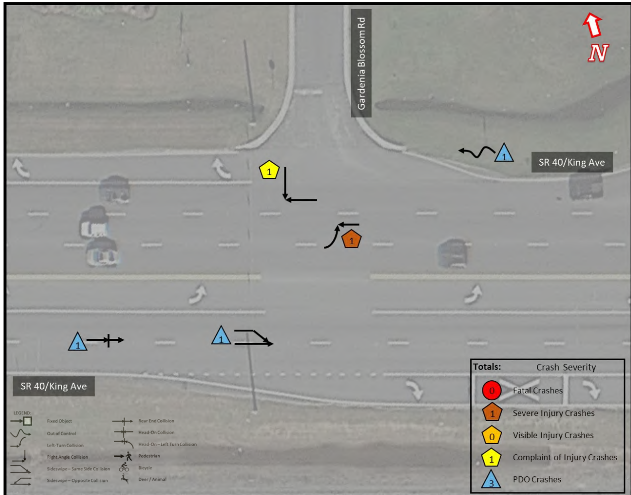
Figure B-5 Crash Diagram for SR 40 at Gardenia Blossom Road Intersection (Jan 1 st , 2013 – February 28th, 2023)
